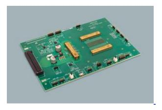
Vicor 1200A LPD solution comprised of an MCD4609 MCM driver and two MCM4609 current multipliers.
