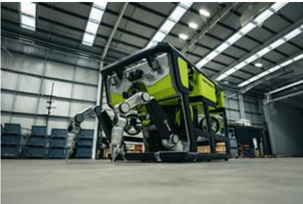
Figure 1 With Vicor's help, Saab has developed the world's most advanced work-class all-electric ROV (eWROV), which combines versatility and maneuverability. Unlike traditional hydraulic ROVs, the eWROV all-electric system eliminates the need for large amounts of hydraulic fluid, thereby mitigating environmental risks.
