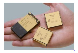
The Vicor automotive-grade power modules for 48V EV systems deliver industry-leading power density and will support automotive OEM and tier one production in 2025. These modules solve complex conversion challenges with 800V, 400V, 48V and 12V systems.
