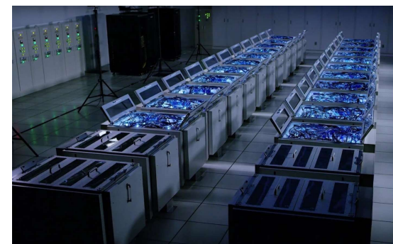
Proof of Concept: PEZY / Exascale Supercomputer (Immersion)
